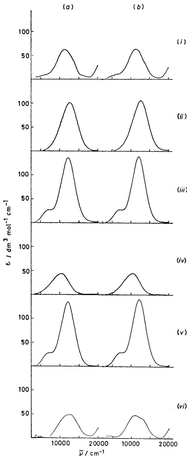
FIGURE 2 Absorption spectra of copper(II) complexes formed by tame (a) and tamp (b) in  $0.5 \text{ mol dm}^{-3} \text{ K}[\text{NO}_3]$ . Species: (i)  $[\text{Cu}(\text{OH})\text{L}]^+$ ; (ii)  $[\text{CuH}_2\text{L}_2]^{4+}$ ; (iii)  $[\text{CuHL}_2]^{3+}$ ; (iv)  $[\text{CuHL}]^{3+}$ ; (v)  $[\text{CuL}_2]^{2+}$ ; (vi)  $[\text{CuL}]^{2+}$ .
