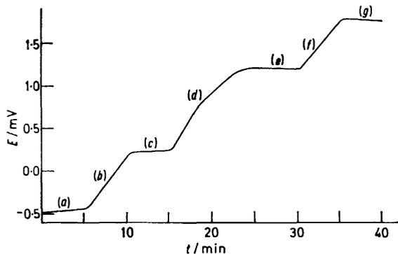
FIGURE 1 Voltage-time plot obtained from a typical calorimetric measurement. For steps (a)—(g) see text
