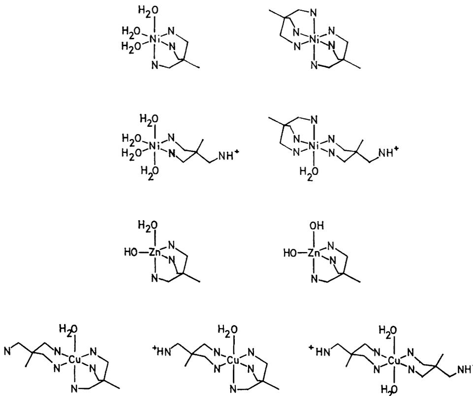
FIGURE 3 Schematic representation of the suggested structures for the metal complexes of tame and tamp
